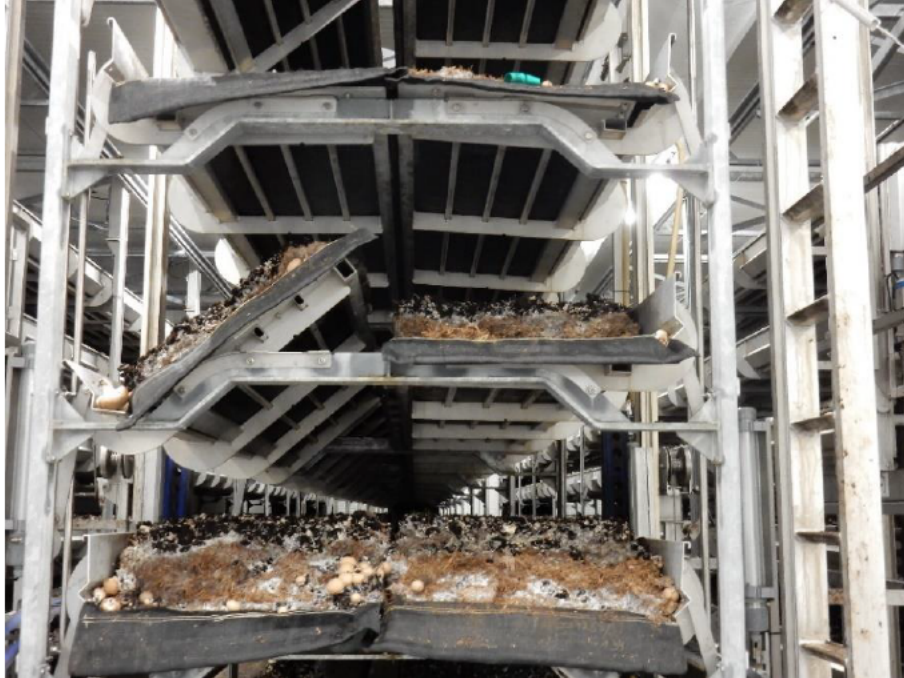
Figure 22. Tilting shelf system - the left side of the second shelf is tilted for harvesting while the other shelves remain flat until ready to harvest.
