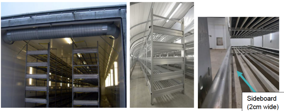
Figure 2. Examples of Dutch shelving in mushroom tunnels.
