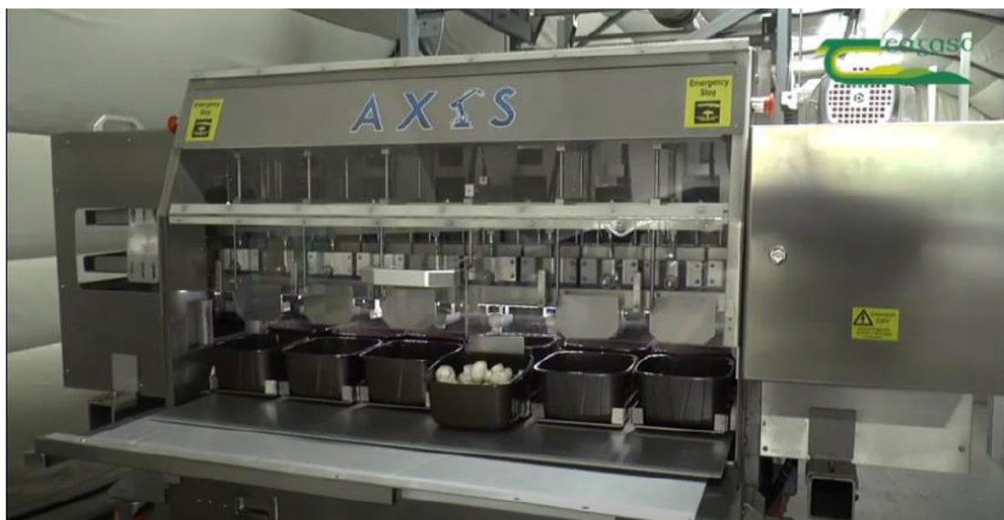
Figure 25. The Axis mushroom processing unit.
