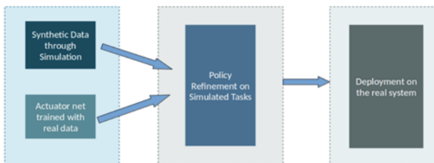
Figure 4.14. Real2Sim Learning SoftGrip actuation dynamics. Incorporation of learned actuator dynamics into the learning pipeline.
