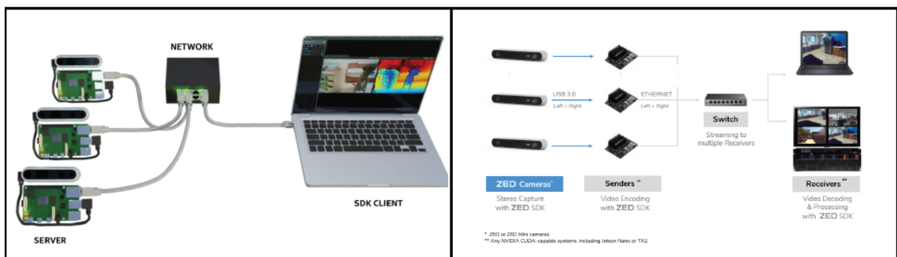
Figure 3.5. The RealSense cameras are connected via USB 3.x to a local SBC which will perform all the processing needed to transfer the camera frames over the network to the main PC.
